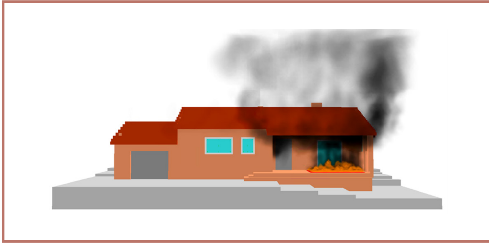
Figure 6: Fire Dynamics Simulator (FDS) analysis of a house with failure of porch window. SOURCE: Dr. Eulàlia Planas, Polytechnic University of Catalonia
